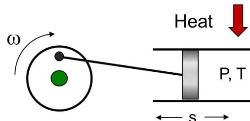
Heating the gas while compressed will raise pressure
