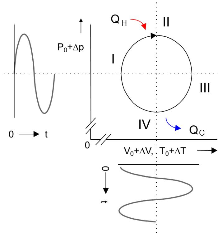
Timing (phase) between pressure, gas displacement and temperature is set by the local complex acoustic impedance inside the regenerator and the thermal response time.
