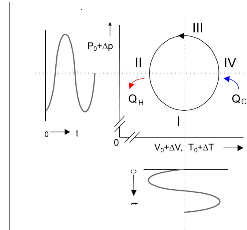
Timing (phase) between pressure, gas displacement and temperature is set by the local complex acoustic impedance inside the regenerator and thermal response time
